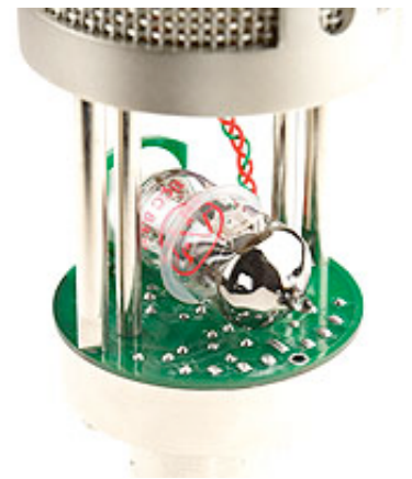
The ECC83 dual triode tube, used in both mics, is fitted to a ceramic base, with the
